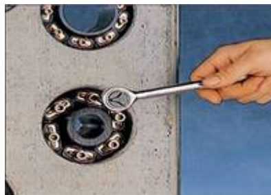
Hexagonal socket head bolts facilitate the assembly of small seal-rings
