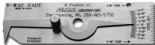
Undercuts/Pits to 1/4 Inch, Crowns to 1/4 Inch by 1/64 Inch Increments (Tolerance .006"). Check Undercuts/Pits, Porosity, Crowns, All Stainless Steel.
